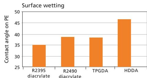
Best wetting of non-polar surface as 100% on corona treated PE with R2395DA compared to any other difunctional monomers – higher non-polar dispersing surface energy
