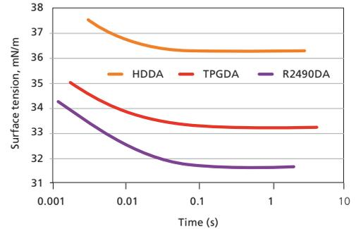
Much lower surface tension for better wetting of low surface energy substrates and pigments with R2490DA vs. hexane diol diacrylate (HDDA) and tripropylene glycol acrylate (TPGDA)
