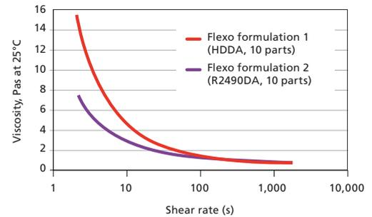
Lower viscosity at lower shear rate for improved flexo ink transfer and flow with R2490DA vs. HDDA
